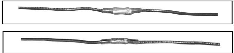
Use a standard crimp tool to crimp the wires in the connector, then use a heat gun to shrink the plastic ends of the connector to seal them.
