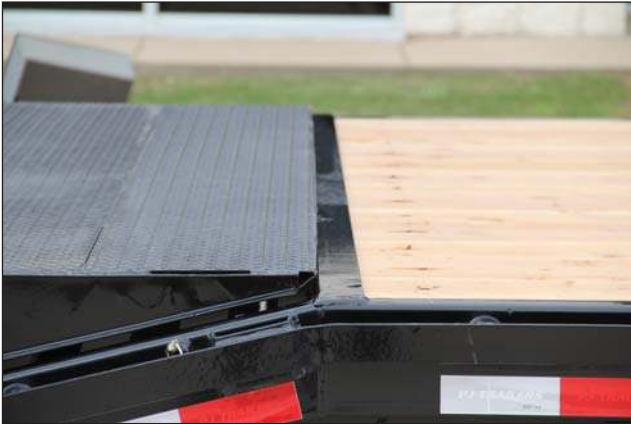
Tail Folded Flat for Storing Cargo
