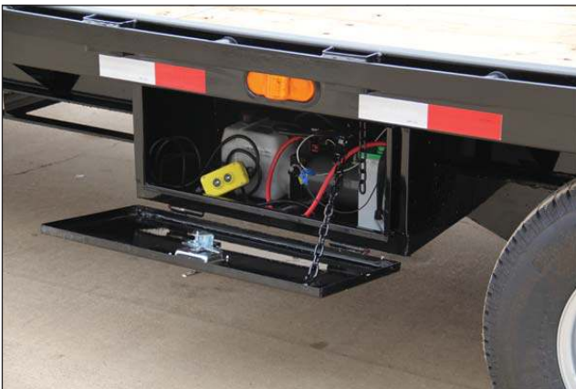
Self-contained Hydraulic Pump System
