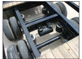
TRAILER FLEX TrailerFlex Air Ride Suspension
